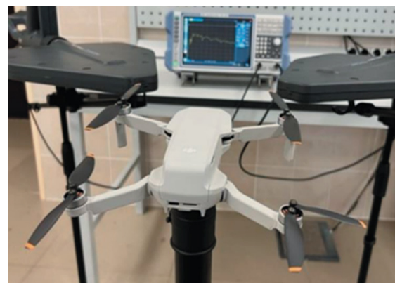
Fig. 1. Quadcopter-type SSO when capturing a radio image
