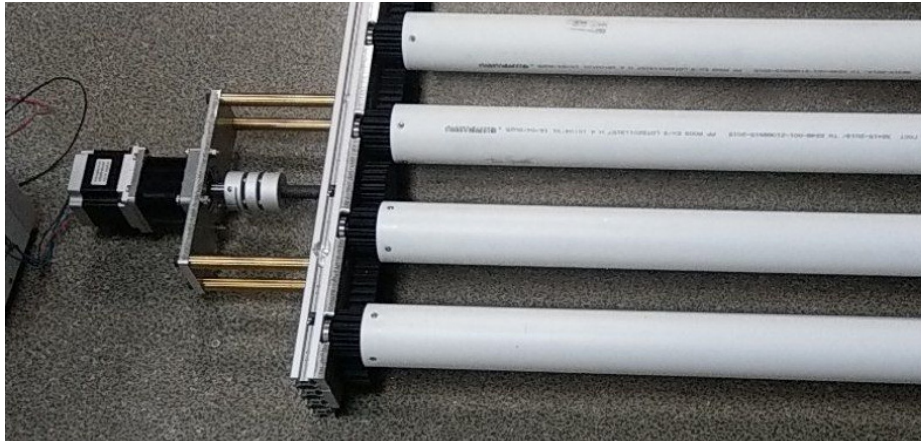
Fig. 5. Mounting the motor via a plate allows it to be adapted to any pitch of the main rollers
