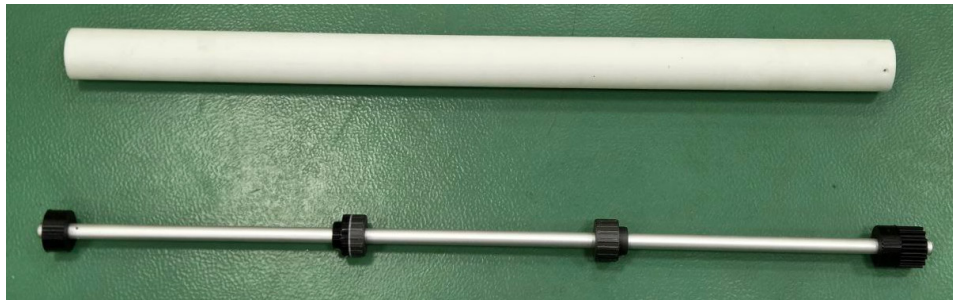
Fig. 3. Main roller shaft with stiffeners, flange, and pulley installed, along with the outer pipe prior to assembly
