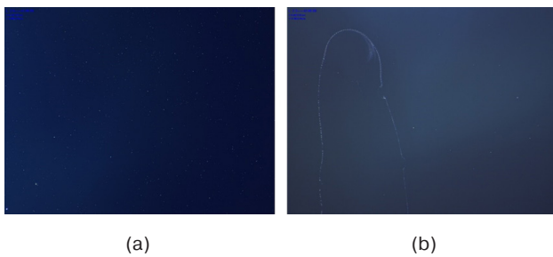
Fig. 7. Si surface after automated cutting: (a) without photoresist, (b) with photoresist. Image at magnification 2.0, field of view area 2.21 \times 2.21 \mu\text{m}^2
