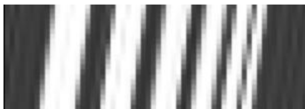
Fig. 13. Blurred picture of a test image with uncropped edges, restored with an inverse filter using the Kotelnikov kernel and no regularization
