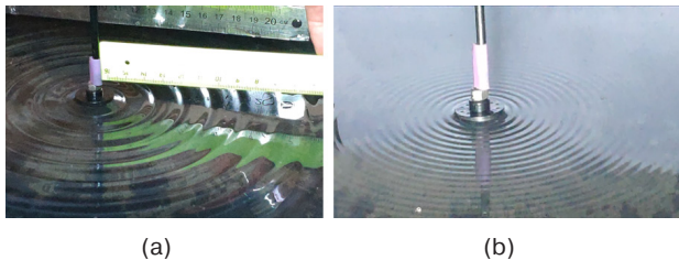
Fig. 2. Images of surface waves at generation frequency f = 16 Hz (a) and at f = 60 Hz (b)
