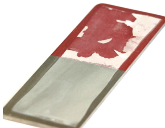
Fig. 1. Photograph of a sample after scale formation testing. The upper part of the sample is protected by a polymer coating
