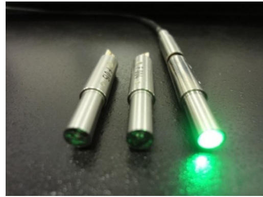
Fig. 5. Specially designed secondary reference LEDs
