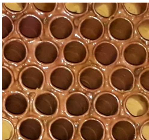
Fig. 2. Appearance of a protective coating on a part of the tube sheet and on a bundle of painted tubes of the horizontal network water heater at the Khabarovsk TPP after 7 months of operation
