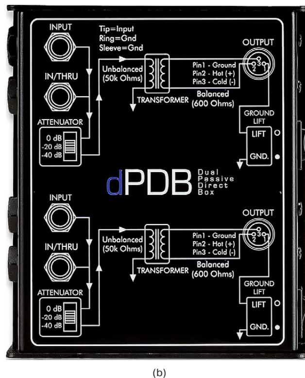
Fig. 6. Mono-balanced implementation of TRS-connector audio routing: (a) in-circuit return/send audio line (with built-in balanced audio device circuit at the input/output); (b) embedding an intermediate analog Di-Box transformer in the line with the ability to select (switch) the ground of the source (audio mixer) or receiver (audio monitor, etc.) [6]
