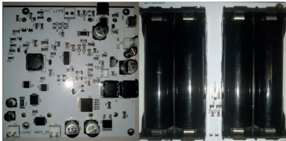
Fig. 13. Prototype for the battery charging and protection unit: top and bottom views
