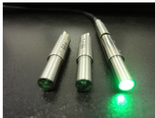
Fig. 5. Specially designed secondary reference LEDs
