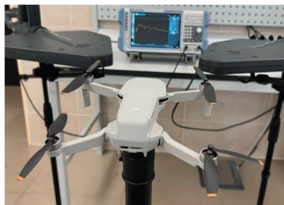
Fig. 1. Quadcopter-type SSO when capturing a radio image
