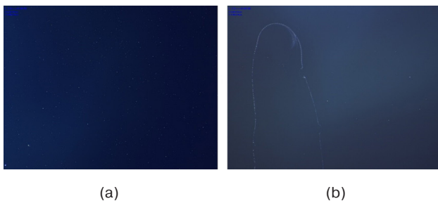
Fig. 7. Si surface after automated cutting: (a) without photoresist, (b) with photoresist. Image at magnification 2.0, field of view area 2.21 \times 2.21 \mu\text{m}^2
