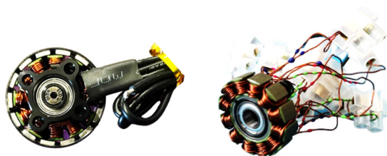
Fig. 1. BLDC motor 2806 + 1350kV before rewinding (left) and after rewinding with the rotor removed (right)
