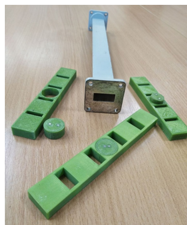
Fig. 2. General view of the manufactured photonic crystals with defect
